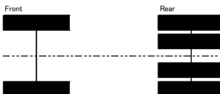
6 x 2 (Front 2 Shaft · Rear 1 Shaft / 1 Shaft Drive)
